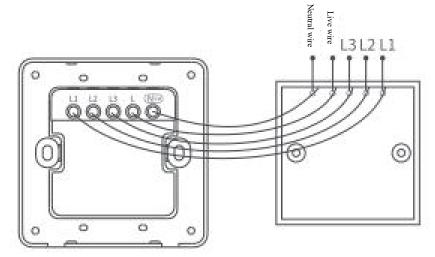
3 Mount the switch on the junction box on the wall with provided screws, and then snap on the switch panel. Make sure to follow the fastening methods to install the panel and the base.
